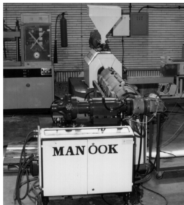
Figure 3. Shear head coupled with single screw extruder.
