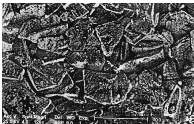
Figure 3. SEM of NdFeB powder with particle size range of 74-100 \mu\text{m} .
