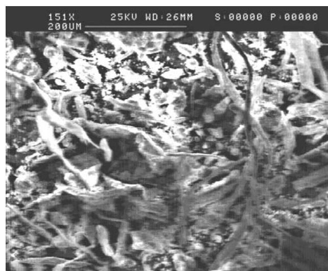
Figure 4. Scanning electron micrograph of paper sludge at magnification 151X.
