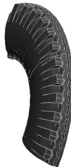
Figure 1. A 3D CAD generated of the 12-24 truck tyre with semi rib tread pattern.
