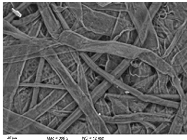
(a) Paper sized with 0.5% cationic starch
