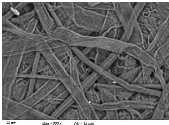
(a) Paper sized with 0.5% cationic starch
