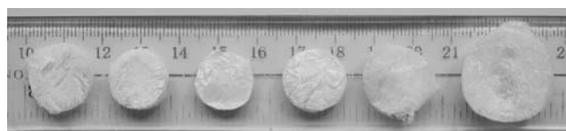
Figure 3. Freeze-dried P(NIPAAm- co -IA) hydrogels (from left to right: G8000, G7505, G7010, G6515, G6020, and G5030, respectively).
