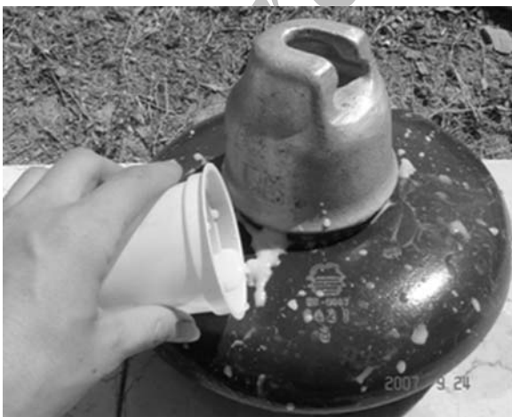
Figure 2. Applying the contamination slurry on insulator.
