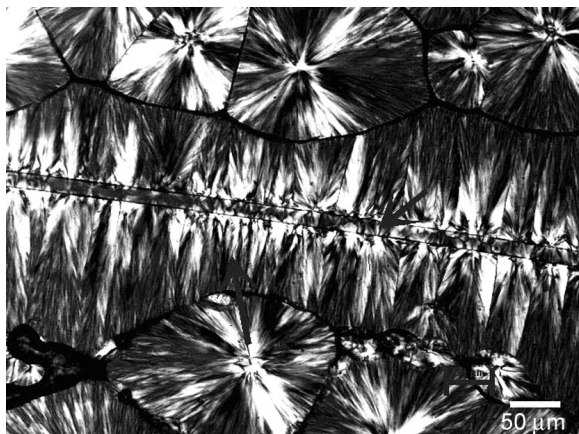
Figure 1. Optical micrograph of the border in glass fibre/polypropylene with isothermal crystallization at 135°C.
