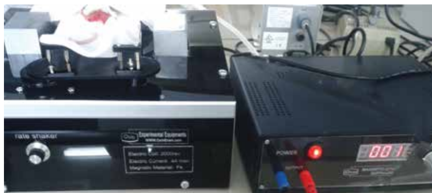
Fig.1: Image of the static magnetic field generating system. Vitrified-warmed ovaries were transplanted into the testicular tissue and the transplantation site was then exposed to a magnetic field for 10 minutes (VOT + group).
