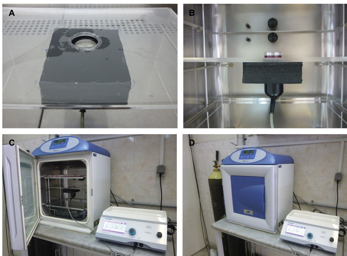
Fig.1: Experimental set-up of the ultrasound-mediated spermatogonial stem cells (SSCs) stimulation. A, B. Position of ultrasound transducer and cell culture plate, C, and D. Orientation of ultrasound stimulation set-up in incubator.
