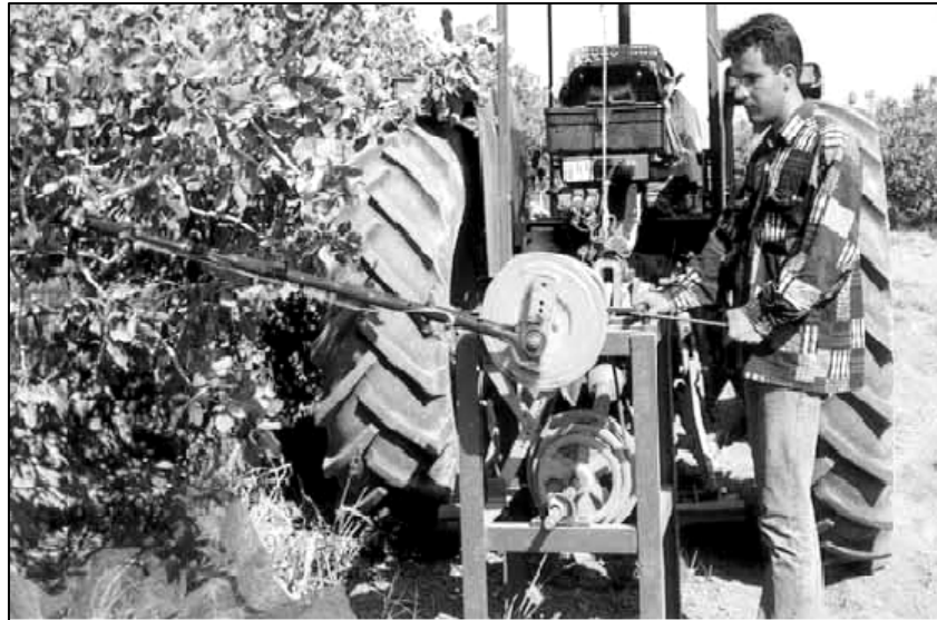
Figure 1. The tractor-mounted limb shaker with adjustable shaking frequency and amplitude
