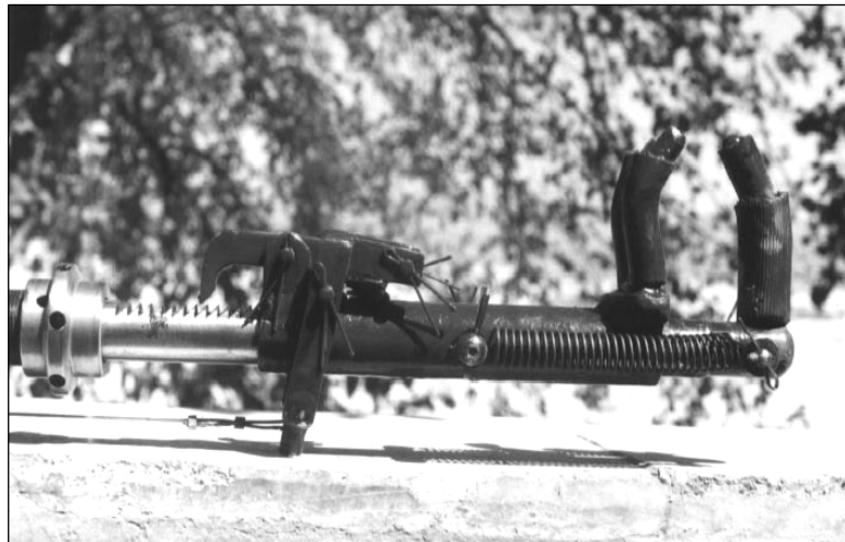
Figure 2. Self-locking gripping fingers of the shaker boom
