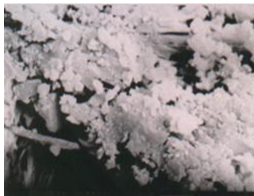
Fig. 2: SEM micrograph of Secar71 hydrated for 9 days at 28 °C ----- 3um.
