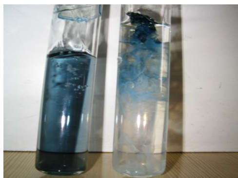
Fig. 5: Effect of divalent cations on gel property, Leading to high degree of syneresis (right) and no syneresis (left).
