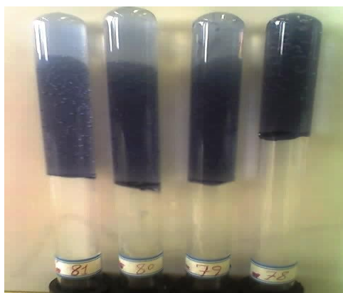
Fig. 8: Effect of water formation on gel polymer properties after 6 hours aging at the reservoir temperature.
