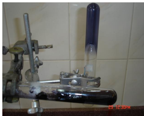
Fig. 4: Effect of excess crosslinking concentration on gel polymer network strength, leading to phase stability (Vertical sample) and phase instability (Horizontal sample).
