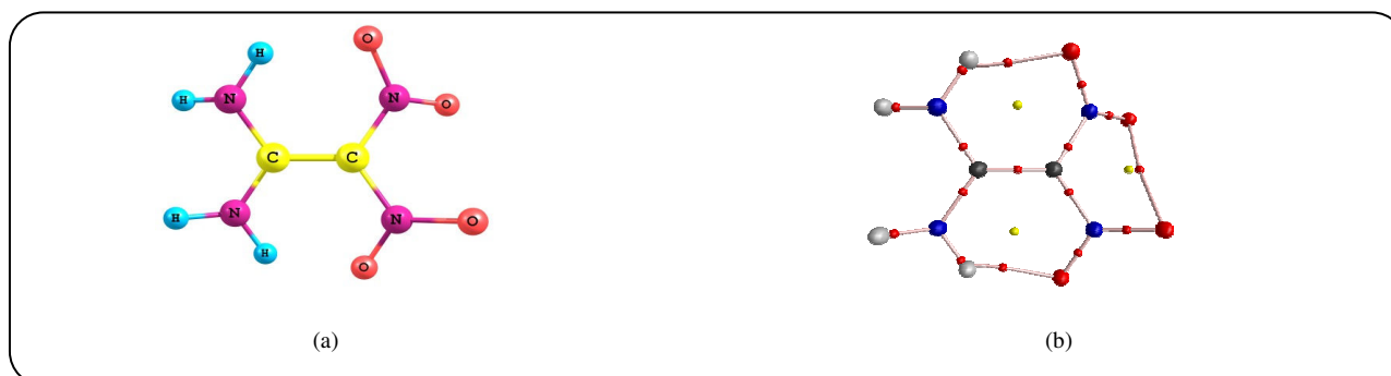
Fig. 1; (a) The optimized geometry of FOX-7 at level of MP2/aug-cc-pVDZ. (b) The 3D molecular graph (MGs) of the equilibrium geometry of FOX-7. (Bold points are Bond Critical Points: BCPs; Pale points are Ring Critical Points: RCPs. The lines are Bond Paths: BPs.)
