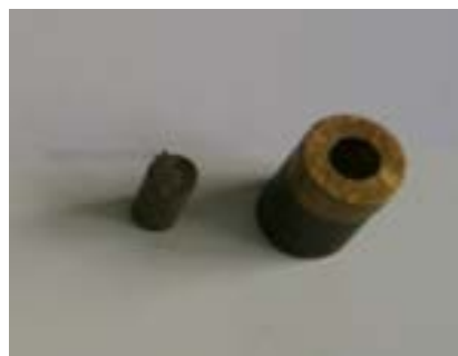
Fig. 2: Casting molds (a): flexural strength (b): compressive strength.
