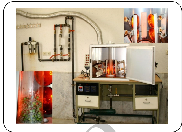
Fig. 2: Fluidized Bed Dryer (FBD) assisted by infrared heating set up.
