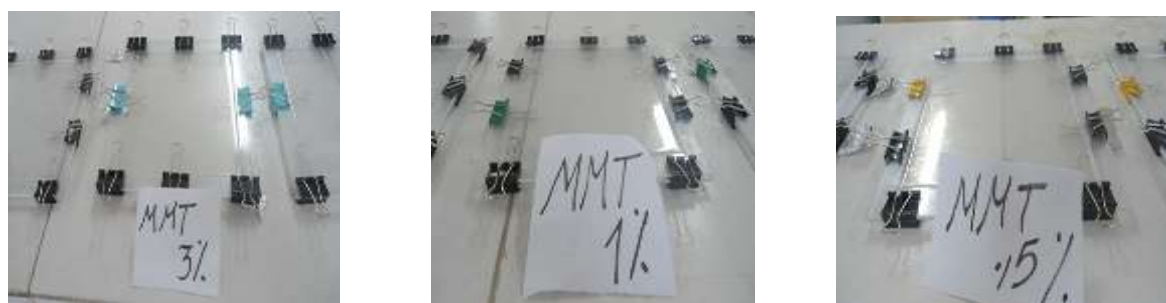
Fig. 1: Prepared CMC/PVA composite films based on different loadings of nanoclay.
