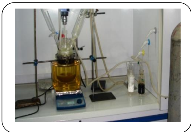
Fig. 1: Experimental set-up for nanocomposite preparation.
