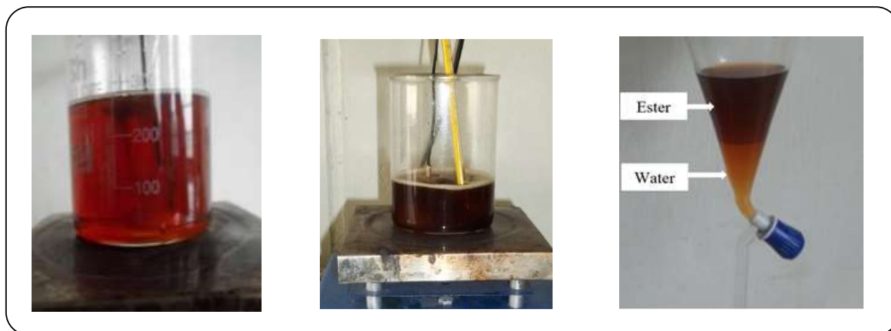
Fig. 4: (a) CD oil, (b) CD oil during esterification, (c) Phase separation after esterification.
