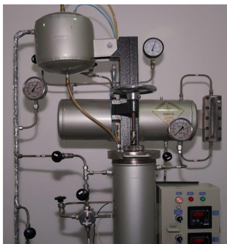
Fig. 1. CO 2 based extractor apparatus.
