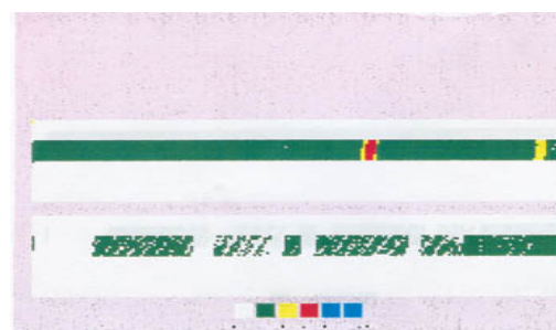
Figure 9. Colored band representing the intensity of applied load on the probe pressure cell.
