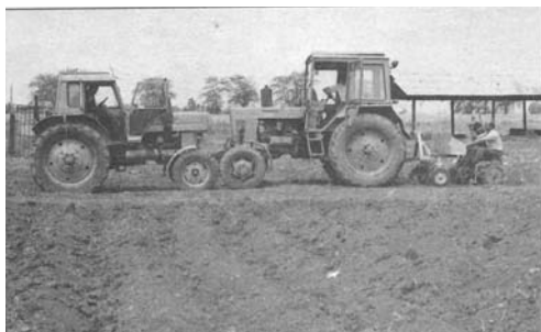
Figure 3. Method of determining required draft.
