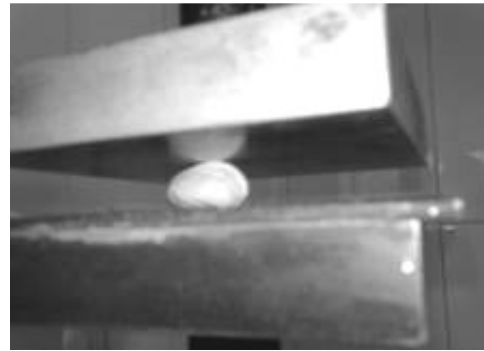
Figure 1. Direction of loading in quasi-static compression test of unsplit pistachio nut using parallel plates.
