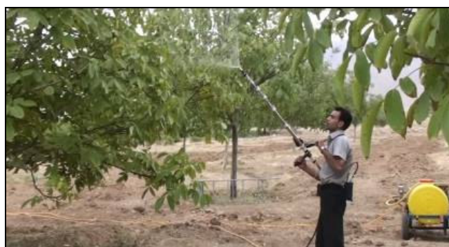
Figure 5. Designed and fabricated telescoping sprayer in operation.
