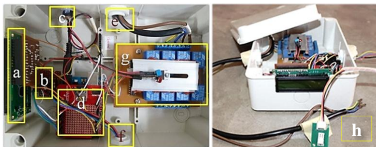
Figure 2. Custom-designed data acquisition system used in data collection with Arduino Uno microcontroller platform.
