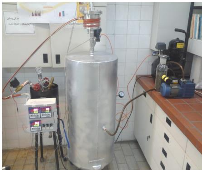
Figure 2. Instant Controlled Pressure Drop (DIC) apparatus. (1) Vacuum Pump; (2) Vacuum tank; (3) DIC treatment chamber; (V1) Steam inlet valve; (V2 and V4) Discharge valve, (V3) Pneumatic vacuum valve.
