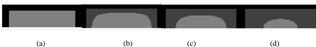
Figure 8. Schematic representation of moisture profile of cellular automata model during hot air drying of banana slice after: (a) 0 (0 s); (b) 20000 (7200 s); (c) 40000 (14400 s), (d) 70000 (25200 S) iterations. Outer rectangular= Drying chamber; Inner rectangular= Banana slice; Black area= Hot air cells; Dark gray area= Dry banana cells; Gray area= Wet banana cells, White area= Dryer tray cells.
