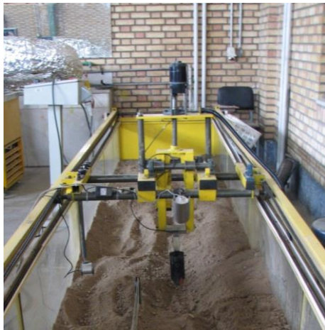
Figure 2. The soil bin used for carrying out the experiment.
