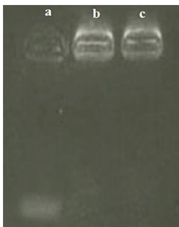
Fig. 6. Confirmation of Apt conjugation. Lane a, un conjugated-MUC1 Apt; lane b, unpurified (NPs + Apt); lane c, purified NP + Apt.
