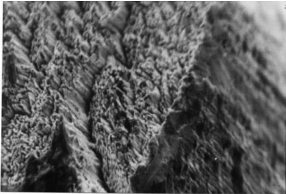
Fig. 9. Pitting corrosion of AISI 1055 in H_2S
