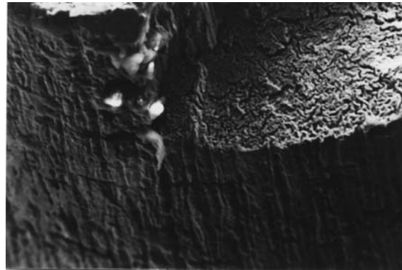
Fig. 10. Initiation of microcracks from surface pits (anodic dissolution)
