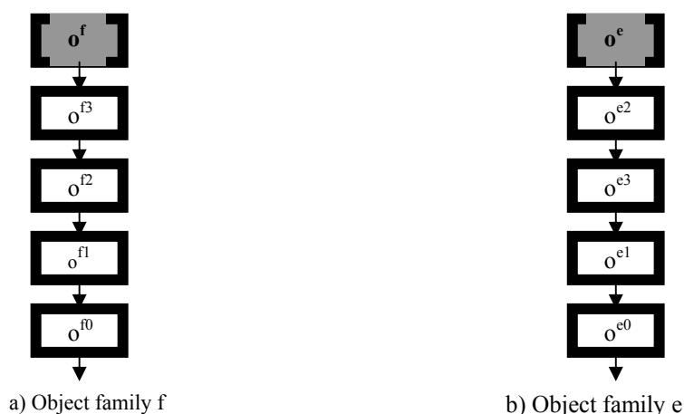
Fig. 7. Example of a possible inter-object serialization Problem
