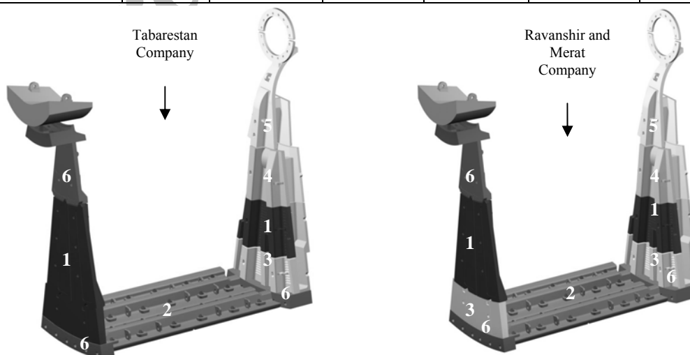
Fig. 9. Ranking of liner/lifter segments according to their wear rates and profiles, wear rates from high to low: 1 (critical), 2, 3, 4, 5, 6
