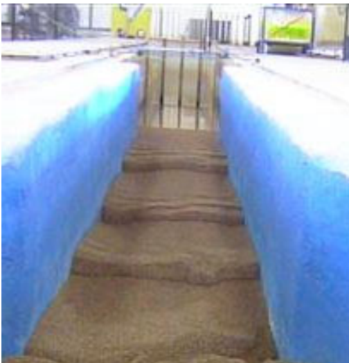
Fig. 3. Dune shape of run 9
