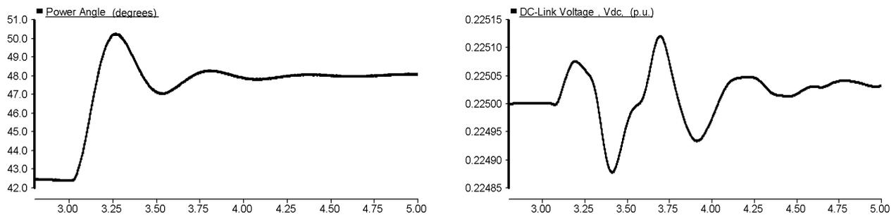
c) The power angle in degrees achieved by MIMO controller      d) The dc-link voltage of the SSSC achieved by MIMO controller
