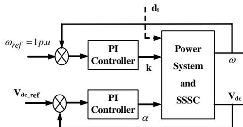
Fig. 5. SISO control system block diagram
