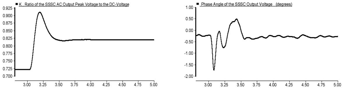
a) The ratio of the ac output peak voltage to the dc voltage of the SSSC      b) The angle deviation of the VSI output voltage
