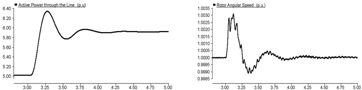
a) The active power transmitted from the line achieved by MIMO controller      b) The rotor angular speed achieved by MIMO controller
