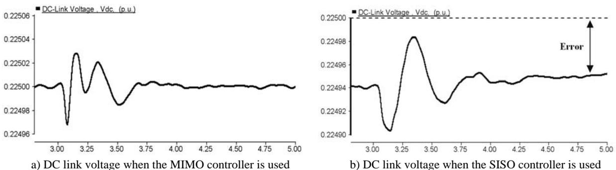
Fig. 9. The dc-link voltage of the SSSC
