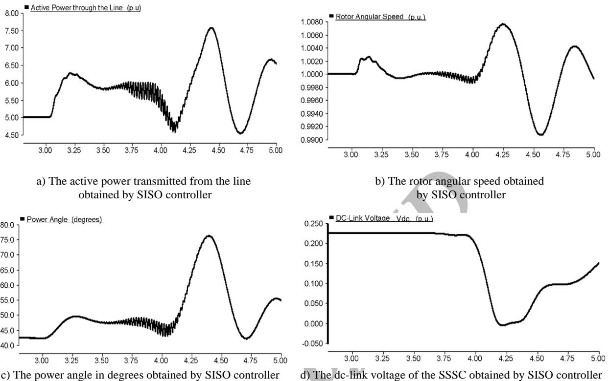
Fig. 12. Simulation results obtained by means of SISO controllers when the operating point is changed
