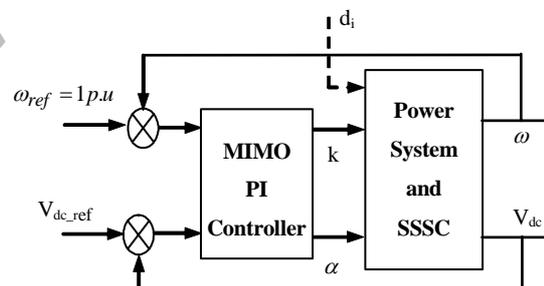
Fig. 3. MIMO control system block diagram
