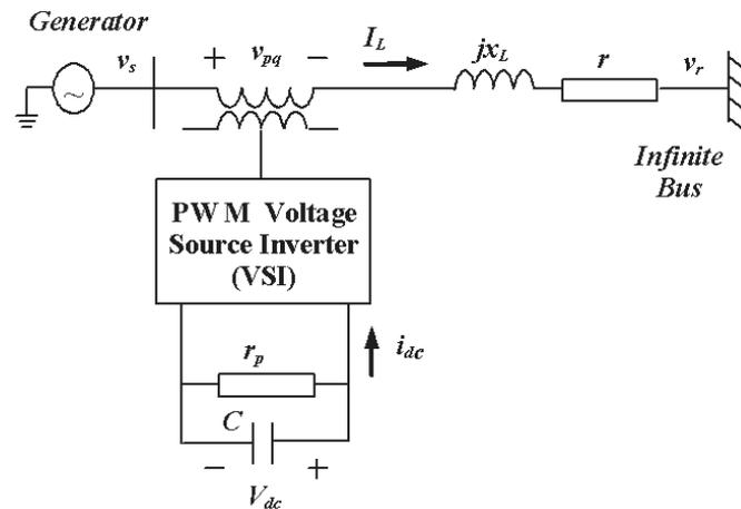
Fig. 1. An SSSC installed in a SMIB three-phase transmission system
