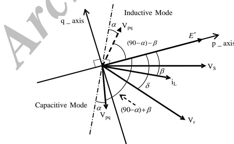
Fig. 2. The phasor diagram of the output voltage of the SSSC for both capacitive and inductive modes
