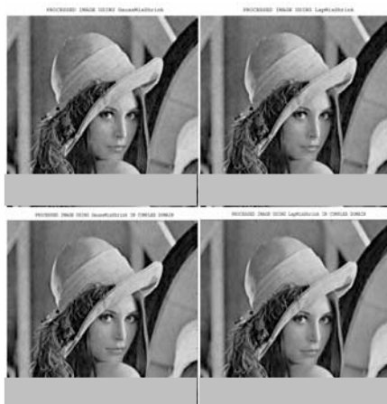
Fig. 16. Denoising with GaussMixShrink and LapMixShrink for Lena image corrupted with additive Gaussian noise with \sigma_n = 20
