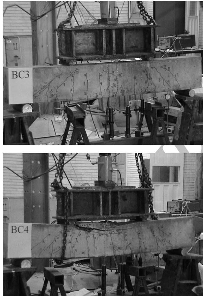
Fig. 2. Crack propagation and failure of the beams under load
