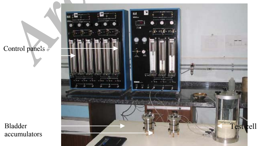
Fig. 2. Triaxial permeability apparatus including the control panels, bladder accumulators, and test cell containing the soil sample
