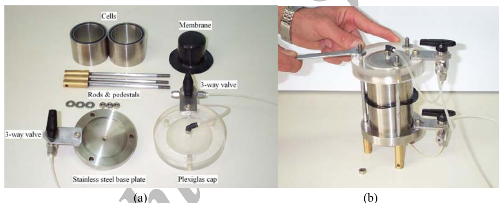
Fig. 1. a) A disassembled bladder accumulator, b) An assembled bladder accumulator
