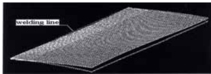
Fig. 23. buckling shape of 3mm shell
