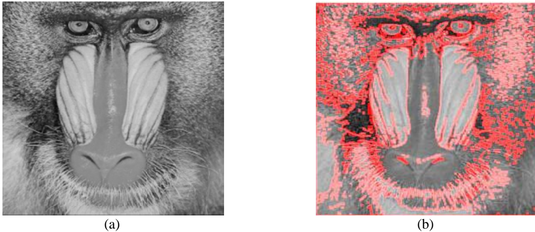
Figure 4. The effect of applying the pixion forming algorithm to the Baboon image: (a) the original image, (b) the output image with boundaries between pixons.
