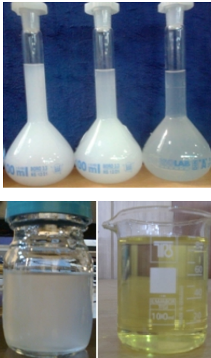
Figure 4. Water (up), EG (left) and transformer oil (right) nanofluid after sonication
