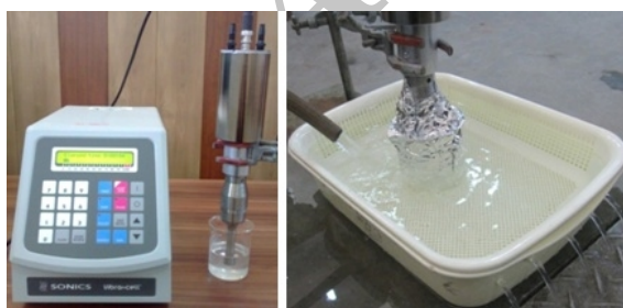
Figure 2. Left: ultrasonic disrupter, right: controlling the suspension temperature
