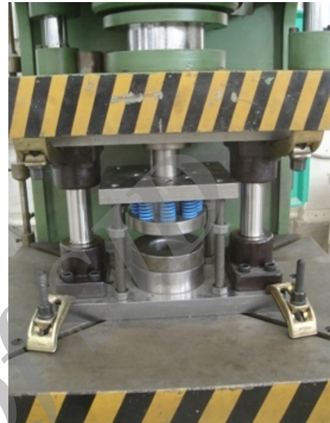
Figure 7. The 60 ton hydraulic press and die set.
