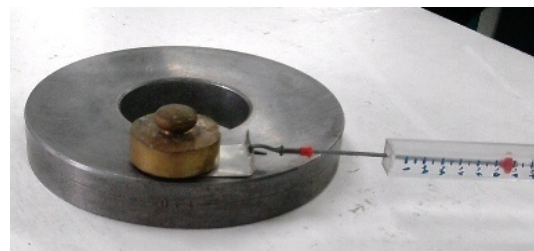
Figure 6. Measurement of friction coefficients
