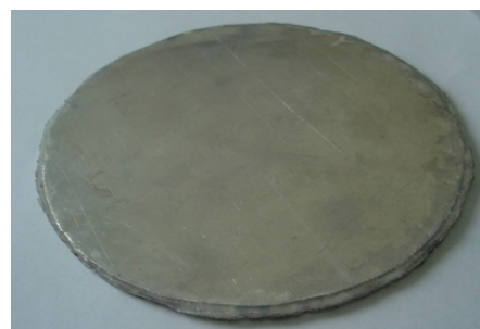
Figure 2. Image of the fiber-metal laminate specimen preparation.
