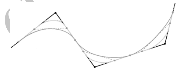
Figure 2. Replacement of an open polygon with two splines which have same sharpness and different expansion.
