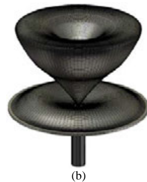
Figure 10. (a) The second optimized profile for UWB monopole antenna with finite ground plane and (b) the 3-D view of antenna
