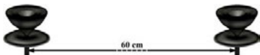
Figure 17. A pair of second optimized antenna placed 60 cm away from each other in free space which are operating as transmitter and receiver
