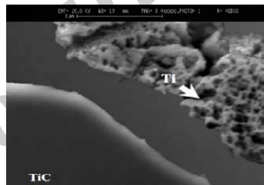
Figure 2. SEM image of Al-6Ti-1C master alloy at 40000X.
