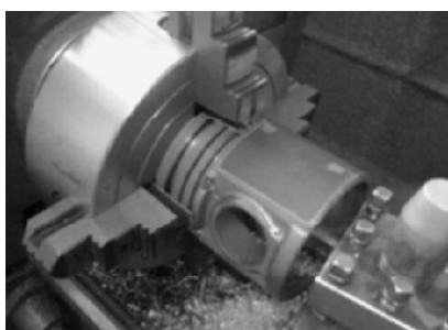
Figure 1. Boring bottom of piston
