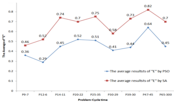
Figure 4. Comparative results obtained for the average of "E" by PSO and SA algorithms
