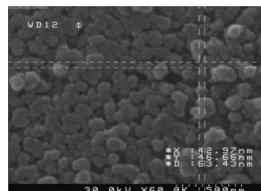
Figure 2. Scanning electron micrographs of sodalite zeolite
