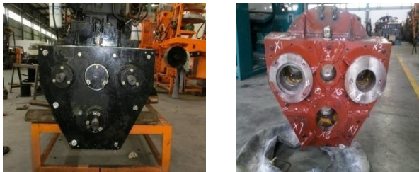
Figure 8. The transfer case before and after improvement
