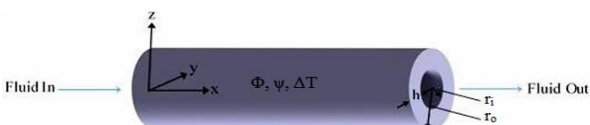
Figure 1. Schematic of fluid-conveying MEE nano-pipe under magneto-electric potential and uniform temperature change.
