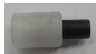
Figure 2. The assembly of the projectile and the sabot
