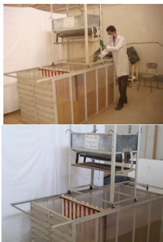
Figure 2. The device used for the reconstitution of specimen
